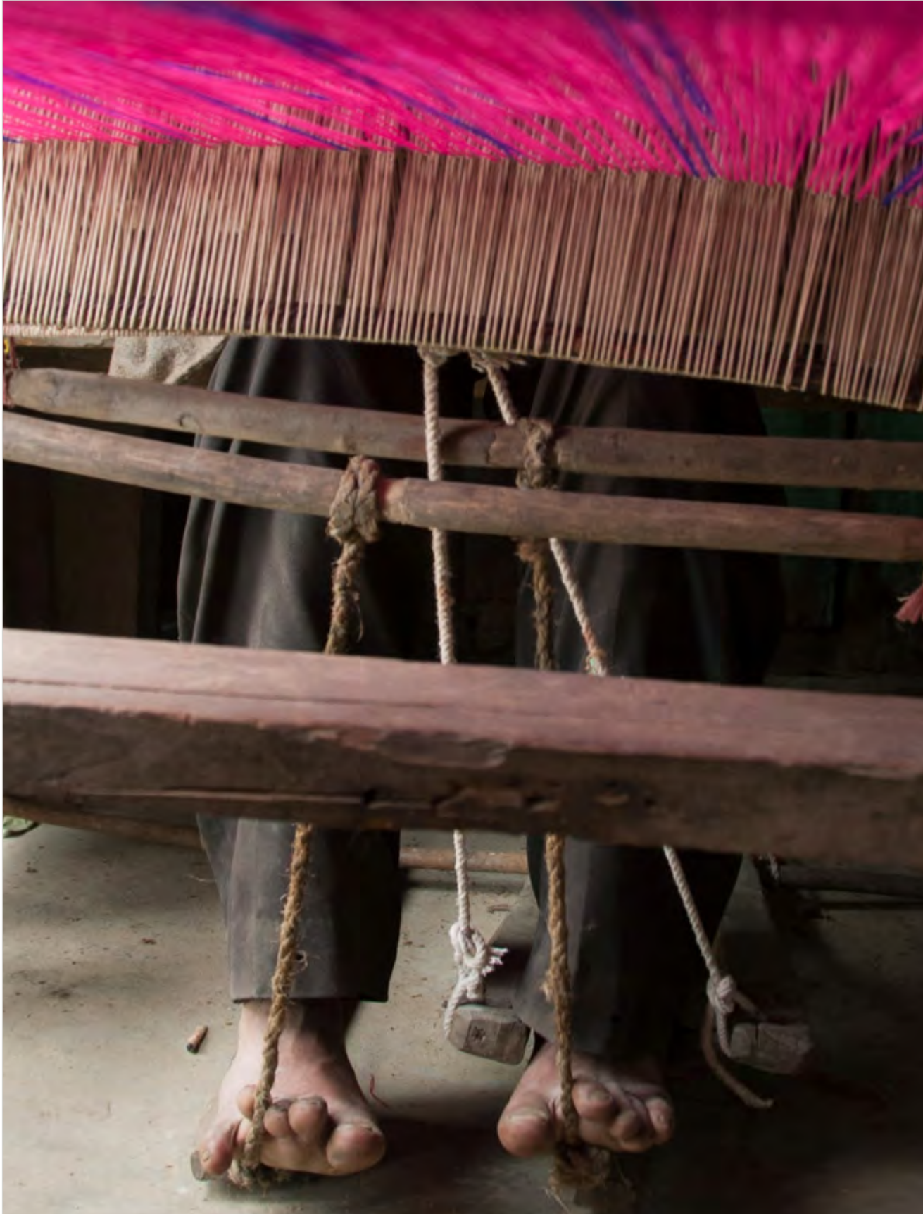
The pedals at the base of the loom, operated by the weaver's feet, determine the plain or diamond weave base of the cloth
